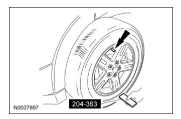
7. Within 2 minutes of the horn sounding, place the Tire Pressure Monitor Activation Tool on the RF tire sidewall opposite (180 degrees) from the valve stem and press and release the test button to train the RF tire pressure sensor.
