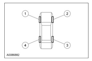
8. **NOTE:** Do not wait more than 2 minutes between training each sensor or the <u>SJB</u> will time out and the entire procedure must be repeated.
